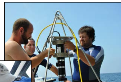
Towfish with sonar used during the 2009 Battle of the Atlantic Expedition All Photos: NOAA
