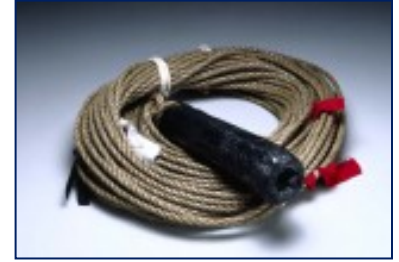
Sounding Lead, 7 lbs, marked in 25 fathom increments (156 feet). Photo: The Mariners' Museum
