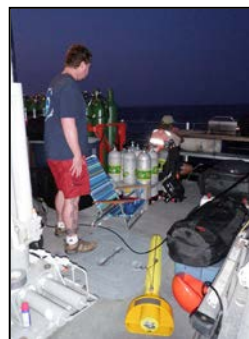
Towfish with sonar used during the 2009 Battle of the Atlantic Expedition All Photos: NOAA
