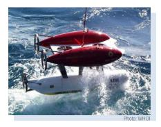
WHOI's Autonomous Underwater Vehicle, the Autonomous Benthic Explorer being deployed
