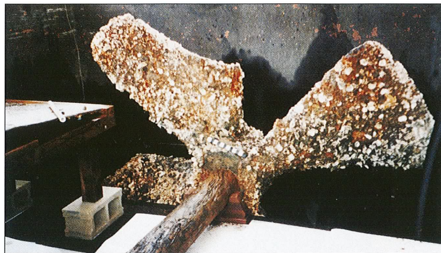
One of the propeller's three broken blades is visible as the propeller sits in the conservation tank during an examination by a conservator (photo courtesy of The Mariners' Museum).
