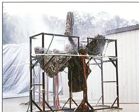
The propeller in its cradle sits under a sprinkler system awaiting conservation at The Mariners' Museum (photo courtesy of The Mariners' Museum).
