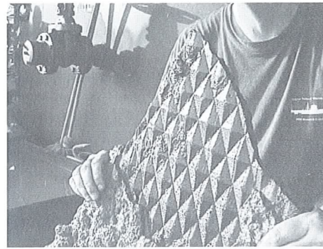
This section of floor plate recovered from the Monitor's engine room has a raised diamond pattern that rendered the surface virtually skid-proof ( Monitor Collection, NOAA).
