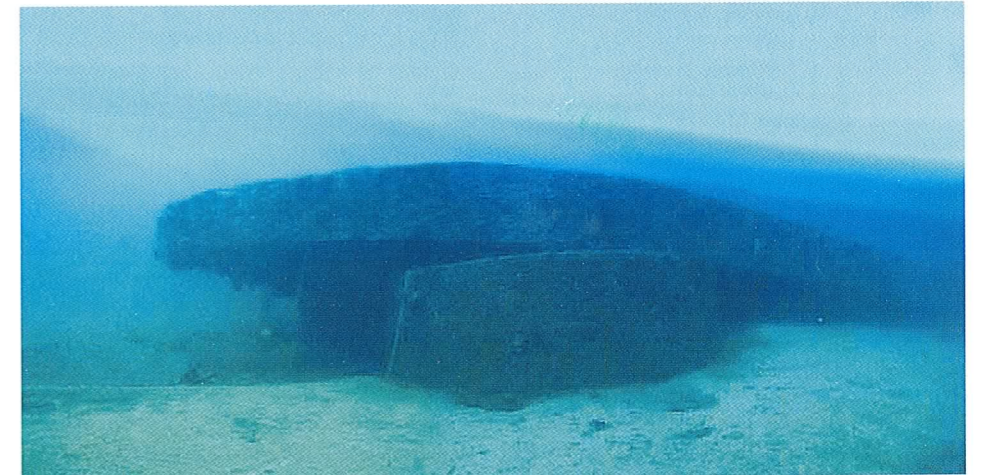
This enhanced photomosaic, made from captured video images, shows the Monitor's stern, port armor belt, and turret. (Jeff Johnston, Monitor Collection, NOAA).
