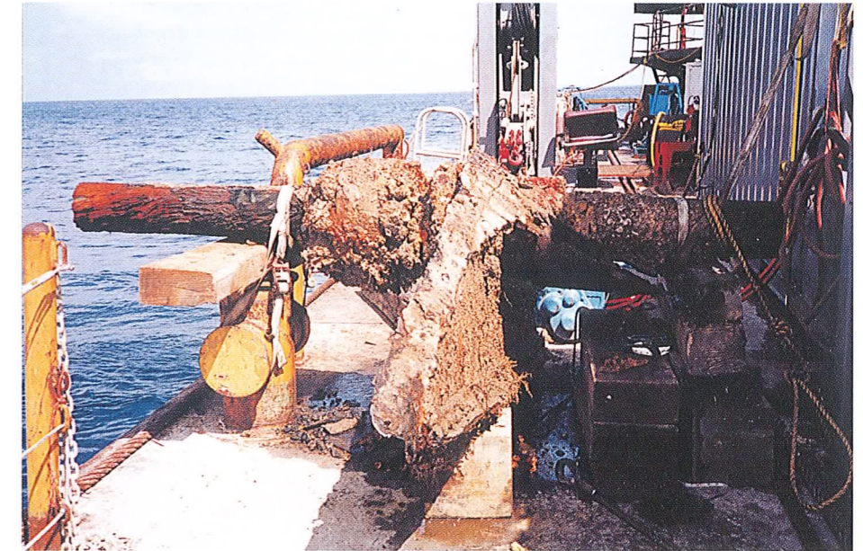
A large section of the Monitor's propeller shaft sits on the deck of the barge following recovery. A section of bulkhead is attached to the shaft (Monitor Collection, NOAA).
