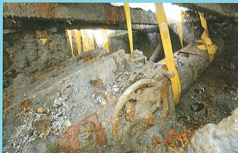
One of the Monitor's two 11-inch Dahlgren guns is shown inside the turret. The Mariners' Museum plans to remove the guns in the near future. Photo: Monitor Collection, NOAA
