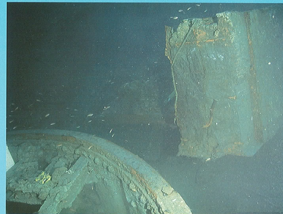
The Monitor's turret was revealed after NOAA and the US Navy removed a 30-ton section of ship's hull and armor belt. Photo: Monitor Collection, NOAA
