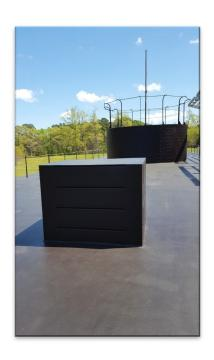
John Ericsson designed the *Monitor* to present the smallest target possible to enemy gunfire. Therefore, most of the ship was below the water, meaning there were no portholes (windows). In order for the captain to command the ship during a battle, he needed to see the action. To allow the captain to view the battle, but remain protected, Ericsson built a small armored pilothouse on the upper deck towards the bow. However, its position prevented *Monitor* from firing her guns straightforward.
