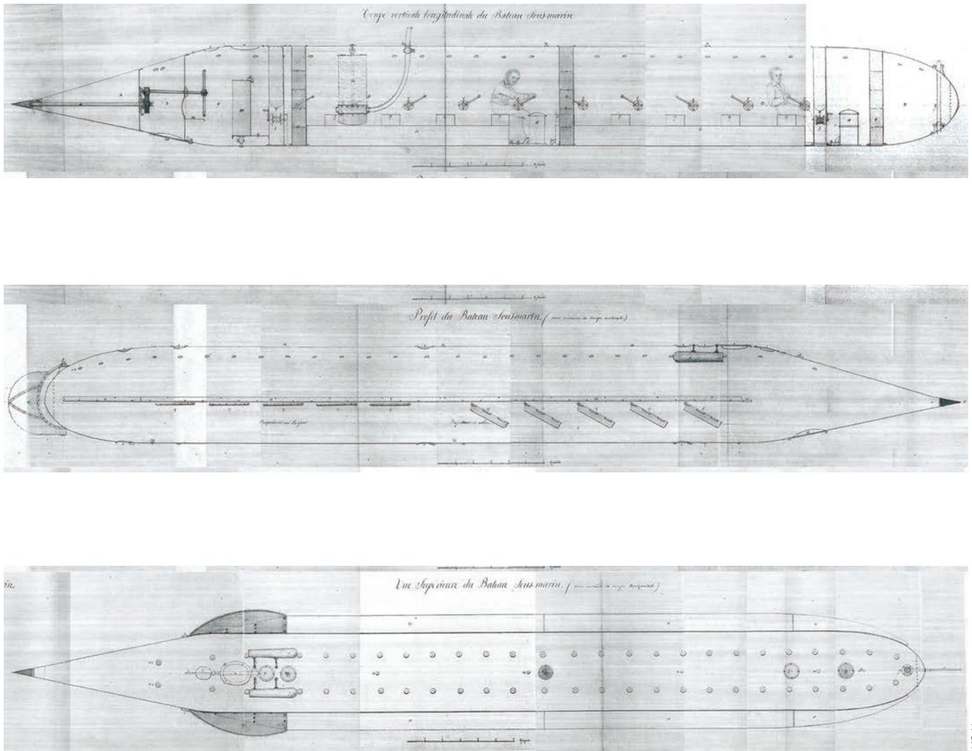
Figure 40. Schematics of USS *Alligator*: The U.S. Navy's first submarine as designed by Brutus de Villeroi, 1863.
