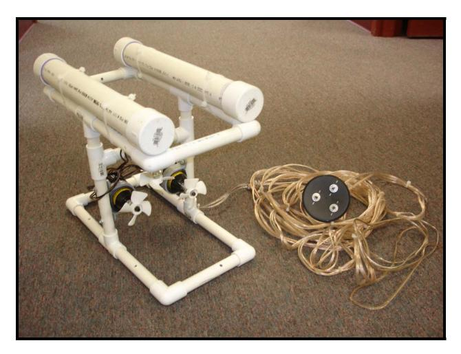
Figure 1.2: This is a side view of an ROV created from parts described in the following pages. The buoyancy pontoons are attached to the PVC frame with plastic tie wraps. A bundle of three pairs of speaker wire transfer the information from the controller jar to the underwater robot.
