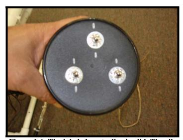
Figure 1.6: The labeled controller jar lid. The silver vertical lines show the direction that the switches can be pushed or pulled.
