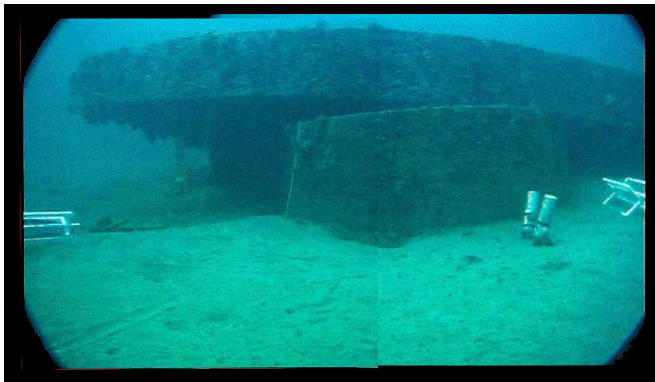
Turret lies upside down under the *Monitor*, also upside down. NOAA installed sacrificial anodes, mounted on PVC frames, to provide temporary corrosion protection for the *Monitor* while recovery planning was underway. Photo: NOAA, *Monitor* Collection
