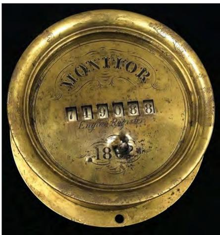
The conserved engine register displays how many hours were on the *Monitor's* engine when the ship sank. Photo: NOAA
